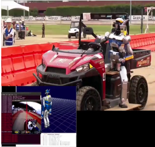
Fig. 4: Humanoid HRP-2 driving a utility vehicle operated by the French-Japanese team in DARPA robotics challenge (© DARPA).
