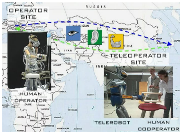
Fig. 3: Intercontinental teleoperation of a humanoid robot executing a collaborative object-carrying with a human.
